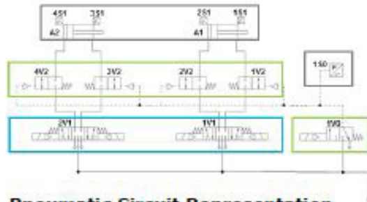
Pneumatic Circuit Representation for CAT 3 Designated Architecture
