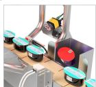
Our reject system tracks product pass signals as they pass the inspection point and uses our patented algorithm to accurately reject products even with continuously varying line speeds.
