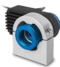
LTPRUP-x models for strobe-only operation featuring ≈ 90W peak power intensity. These models are compatible with CMHO016 clamping mechanics, alternatively three M4 and one M6 threads are available as fixing options.
