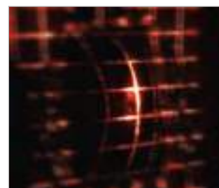
Without tilt adjustment, the image of the surface is not homogeneously focused.
