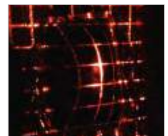
At the Scheimpflug angle, the image is sharp over the entire surface where the paste has been deposited.
