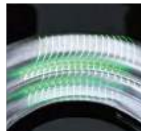
Scheimpflug telecentric optics for both projection and imaging at 90°.
