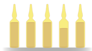
Liquid level inspection.
