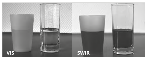
Liquid level inspection.
