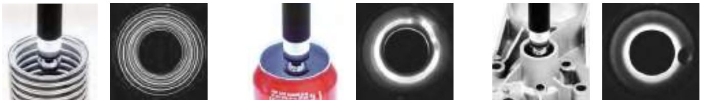
Tube scanning for integrity inspection.
