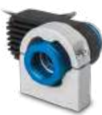
LTPRUP-x models for strobe-only operation featuring ≈ 90W peak power intensity. These models are compatible with CMH0016 clamping mechanics, alternatively three M4 and one M6 threads are available as fixing options.
