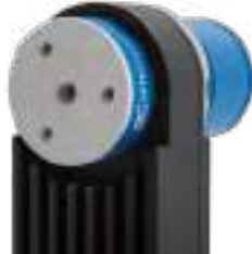
LTPRUP-x models for strobe-only operation featuring ≈ 90W peak power intensity. These models are compatible with CMH0016 clamping mechanics, alternatively three M4 and one M6 threads are available as fixing options.
