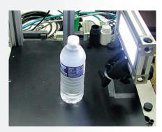
**SOLUTION:** With a backlight placed behind the bottle, the inspection for the bottle cap, fill level, and safety seal are clearly visible to the camera. The system can easily pass correctly fitted caps and proper safety seals, as well as view fill levels. Improperly fitted caps, questionable safety seals, and inaccurate fill levels are failed by the vision system.
