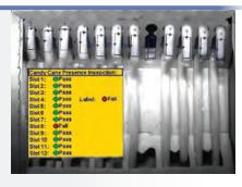
SOLUTION: To combat this variation, Smart Vision Lights recommended infrared (IR) illumination, which is invisible to humans and also eliminates various colors of objects, providing a grayscale image result. IR light is also used to see through packaging to inspect goods since it penetrates plastic wrappings, eliminating any potential for glare or reflection. With the IR light, all the canes appear very bright white. If a cane is missing, the location where it should be appears dark.
