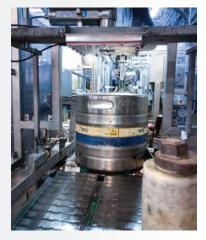
SOLUTION: After implementing an in-line keg inspection system at the production line, the customer was able to detect problematic microleaks, as well as damage or anomalies in keg spears. By detecting and removing faulty products at an early phase, customer complaints decreased by more than 50 percent.
