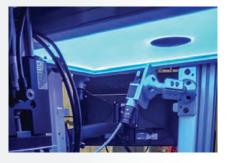
**SOLUTION:** By placing a large, diffused light at 45- degrees to the camera's field of view, a 5-megapixel camera was easily able to differentiate between metal beveled edge and glass panel inside the metal frame. A separate large panel light was used to backlight bowl-fed components, while a third large panel backlight was used to differentiate between a cured glue bead and the glass panel.
