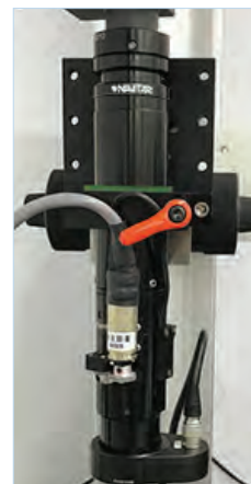
Optotune Module (Navitar 1-64805) with Zoom 6000 Motorized System
