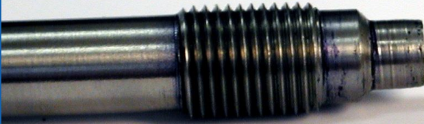
Tip Compression from Bad or Unclean Hole
