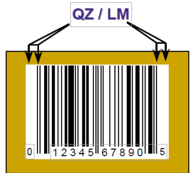
Clear areas around the bar code necessary for the scanner to properly recognize and read the bar code. They are free of wording, graphics, closures, perforations or scores.
