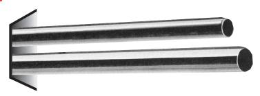
Maximum Working Pressure (PSIG) =  $\frac{2 \times \text{Material Strength (PSI at Room Temperature)} \times \text{Wall Thickness of Tube (in)}}{\text{OD of Tube (in)} \times \text{SF (Safety Factor of 1.5 to 10 depending on application)}}$
