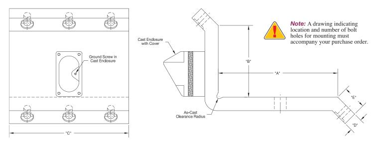
"L" Shaped Cast-In Heaters — 45° Flange Mount Style
