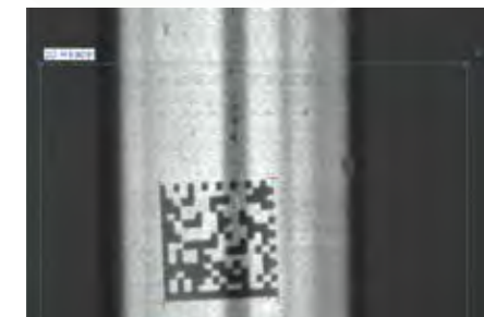
LASER-ETCHED 2D CODE ON METAL
