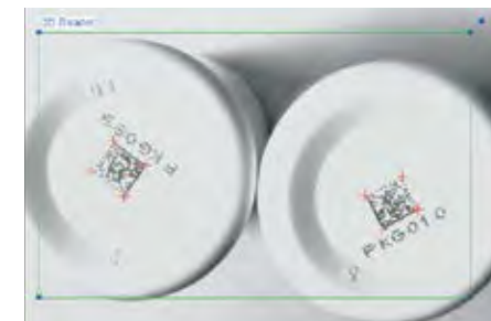
DOT PEEN 2D CODES ON PLASTIC
