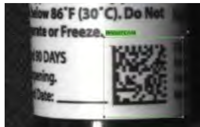
2D CODE PRINTED ON PHARMACEUTICAL VIAL
