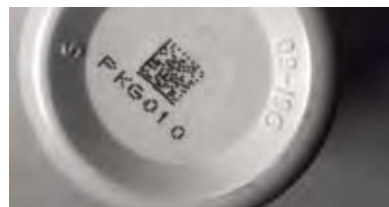
2D CODE PRINTED ON UNDERSIDE OF PLASTIC BOTTLE
