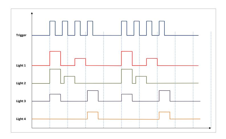
Gardasoft's CC320 trigger timing controller could be used to generate triggers for the cameras and lighting controller and integrate other signals such as part sensor, conveyor belt encoder and reject gate.
