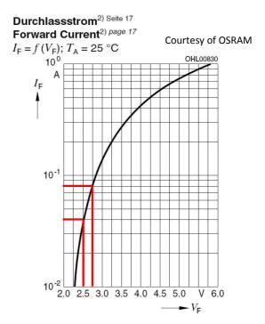
Controlling the current allows for precise control of the LED light output, additional benefit is then also available to users are looking to overdrive their lights to increase light output.
