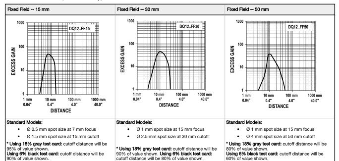
Fixed-field focus and spot sizes are typical. Performance based on use of 90% reflectance white test card.\*
