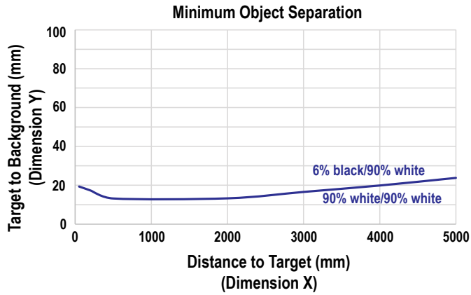
Figure 21. Minimum Object Separation for 250 ms Response Time
